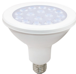
03PAR38-15W/17W Plastic housing+PC cover Wattage: 15W/17W Lumen: 1200lm/1360lm Voltage: AC220-240V 50/60Hz LED Type: 2835 SMD Beam angle: 38°/60° Lamp base: E27 CCT: 2700-6500K PF: 0.5 Size: Dia122xH125mm Lifespan: 25000hrs
