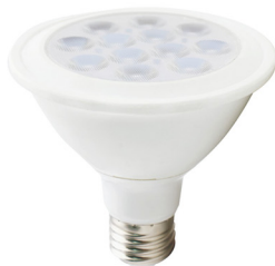
03PAR30-11W/13W Plastic housing+PC cover Wattage: 11W/13W Lumen: 900lm/1000lm Voltage: AC220-240V 50/60Hz LED Type: 2835 SMD Beam angle: 38°/60° Lamp base: E27 CCT: 2700-6500K PF: 0.5 Size: Dia95xH100mm Lifespan: 25000hrs
