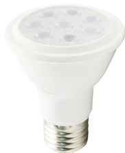
03PAR20-7W/9W Plastic housing+PC cover Wattage: 7W/9W Lumen: 500lm/720lm Voltage: AC220-240V 50/60Hz LED Type: 2835 SMD Beam angle: 38°/60° Lamp base: E27 CCT: 2700-6500K PF: 0.5 Size: Dia63xH82mm Lifespan: 25000hrs
