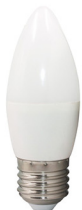
03C37--(3W/5W/6W) Plastic housing+PC cover Wattage: 3W/5W/6W Lumen: 250lm/400lm/470lm Voltage: AC220-240V 50/60Hz LED Type: 2835 SMD Beam angle: 160° Lamp base: E27 CCT: 2700-6500K PF: 0.5 Size: Dia37xH98mm Lifespan: 25000hrs
