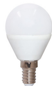
03P45--(3W/5W/6W) Plastic housing+PC cover Wattage: 3W/5W/6W Lumen: 250lm/400lm/470lm Voltage: AC220-240V 50/60Hz LED Type: 2835 SMD Beam angle: 160° Lamp base: E14 CCT: 2700-6500K PF: 0.5 Size: Dia45xH78mm Lifespan: 25000hrs
