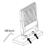
2 Adjust the light angle, fasten the bolt
