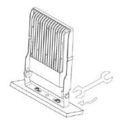
3、 Connect the cord,Note:the terminal shall be waterproof.
